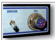
(left) Front Panel with Option 07 showing Key Fill Loader Interface and Zeroize Function
